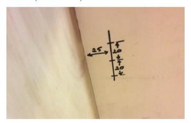
2. Drill pilot holes (4mm) on cross lines
